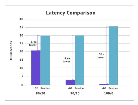
Figure 6: Millisecond Latency at p95 for rDE compared to direct access to Cassandra
