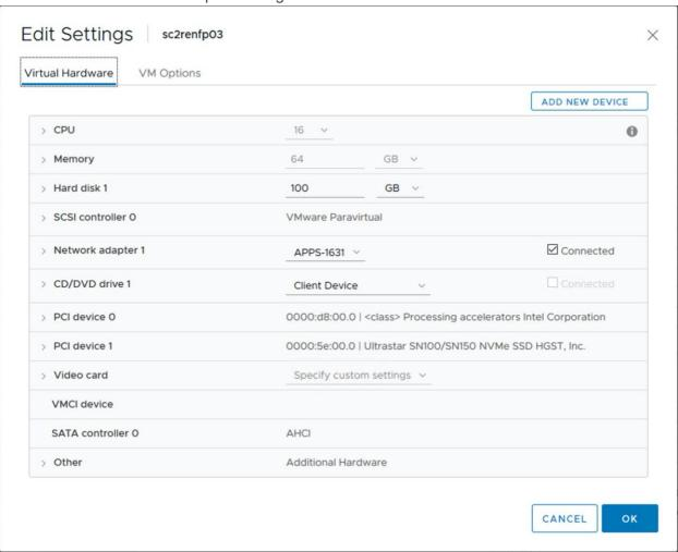
Figure 3: rDE virtual machine settings with passthrough devices
