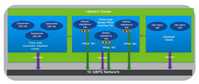
Figure 2: Logical Schematic of Virtualized rDS & Cassandra
