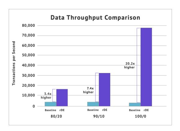
Figure 5: Transactions per second for rDE compared to direct access to Cassandra
