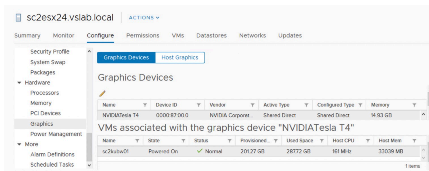
Figure 5: vSphere Node with virtual machines using NVIDIA vGPU
